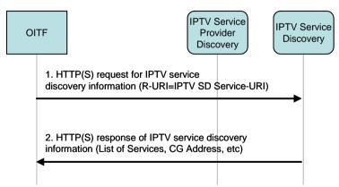
Figure 6-4: IPTV Service Discovery for unmanaged networks
