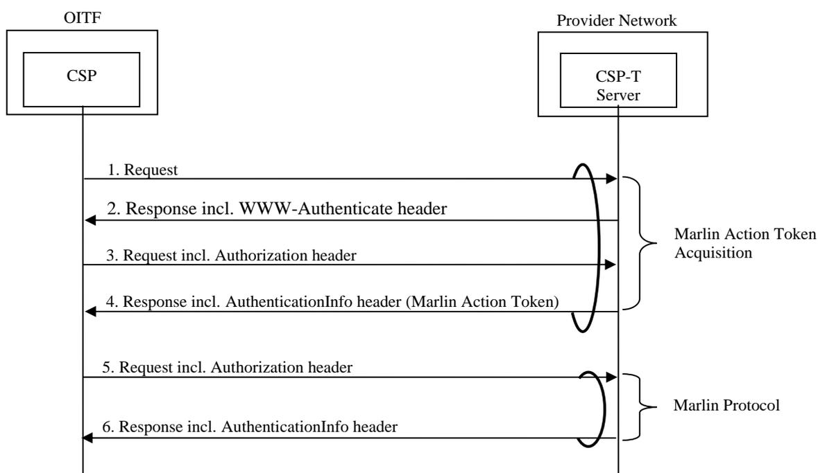
**Figure 33: User Authentication for CSP, CSP-T Server communication**
