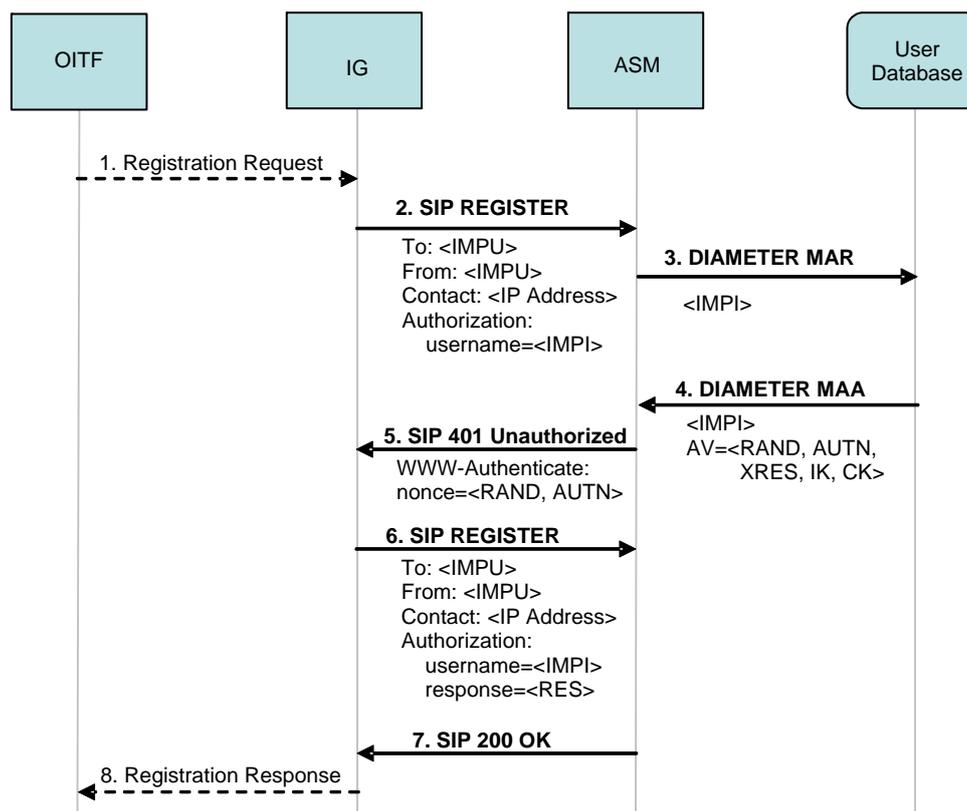
**Figure 28: User Identification and Authentication based on the IMS AKA procedure**
