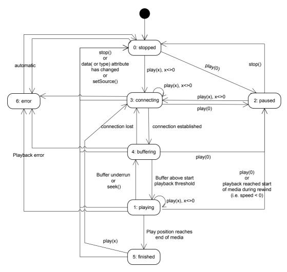
Figure 13: State diagram for embedded A/V Control objects
