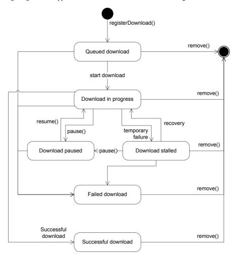
Figure 10: State diagram for embedded application/oipfDownloadManager objects
