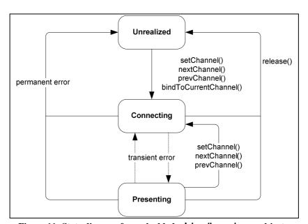
Figure 11: State diagram for embedded video/broadcast objects.
