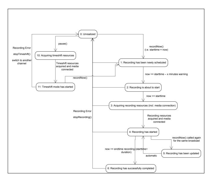
Figure 12: PVR States for recordNow and timeshifting using video/broadcast
