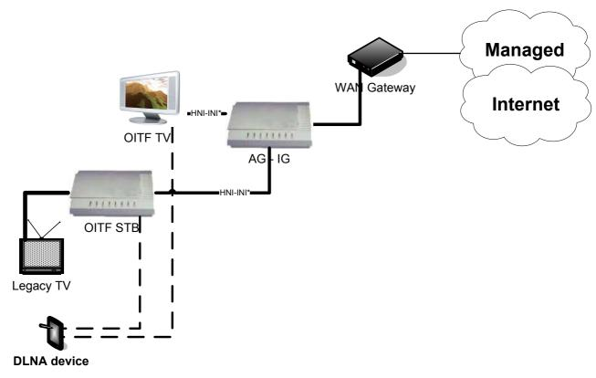
This deployment supports both managed and unmanaged services, with DAE and PAE applications, presented on an OITF TV and a legacy TV. The following devices are deployed:
