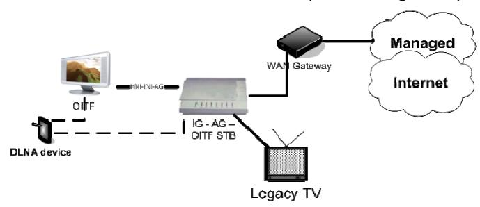
This deployment supports both managed and unmanaged services, with DAE and PAE applications, presented on an OITF TV and a legacy TV. The following devices are deployed:
