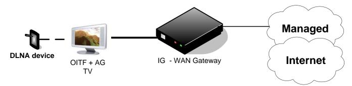
This deployment supports managed and unmanaged services, and DAE and PAE applications. The following devices are deployed:
