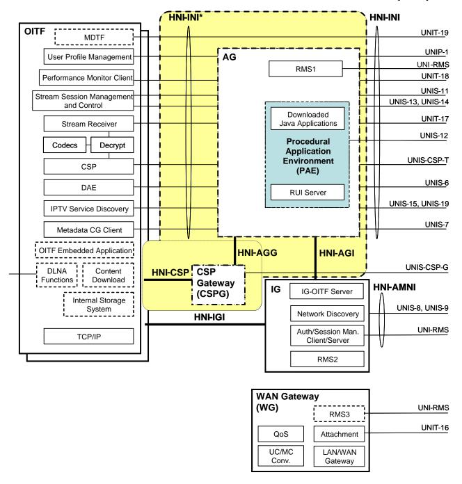
Figure 1: Consumer Network High Level Architecture
