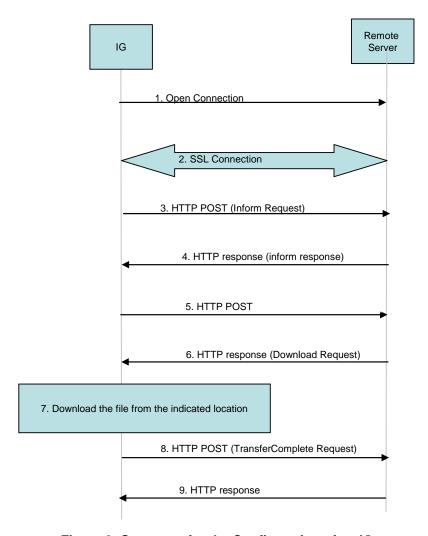
Figure 3: Sequence for the Configuration of an IG
