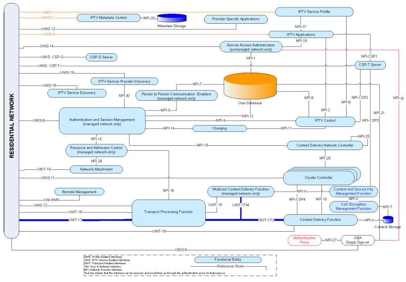
Figure 2: Provider Network High Level Architecture
