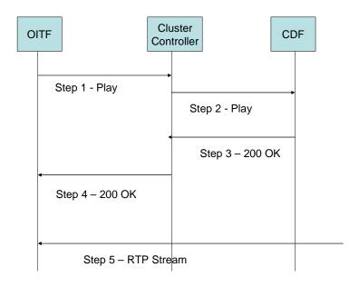
Figure 4: RTSP Procedure on UNIS-11 for managed model
