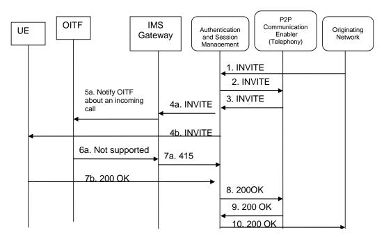
Figure 16: IMS telephony service based caller identification
