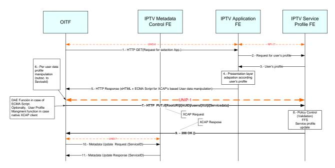
Figure 11: Service Profile Management Based on XCAP
